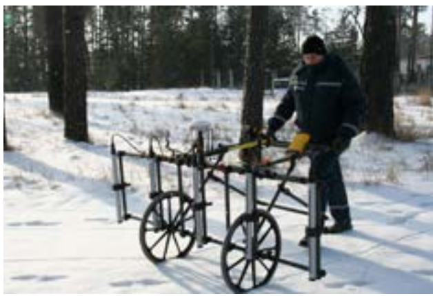
A staff member from the State Emergency Service of Ukraine (SESU) testing a multi-channel unexploded ordnance (UXO) detection system provided within an OSCE FSC Project, 12 December 2016, SESU Training Centre, Kharkiv region, Ukraine (SESU)
