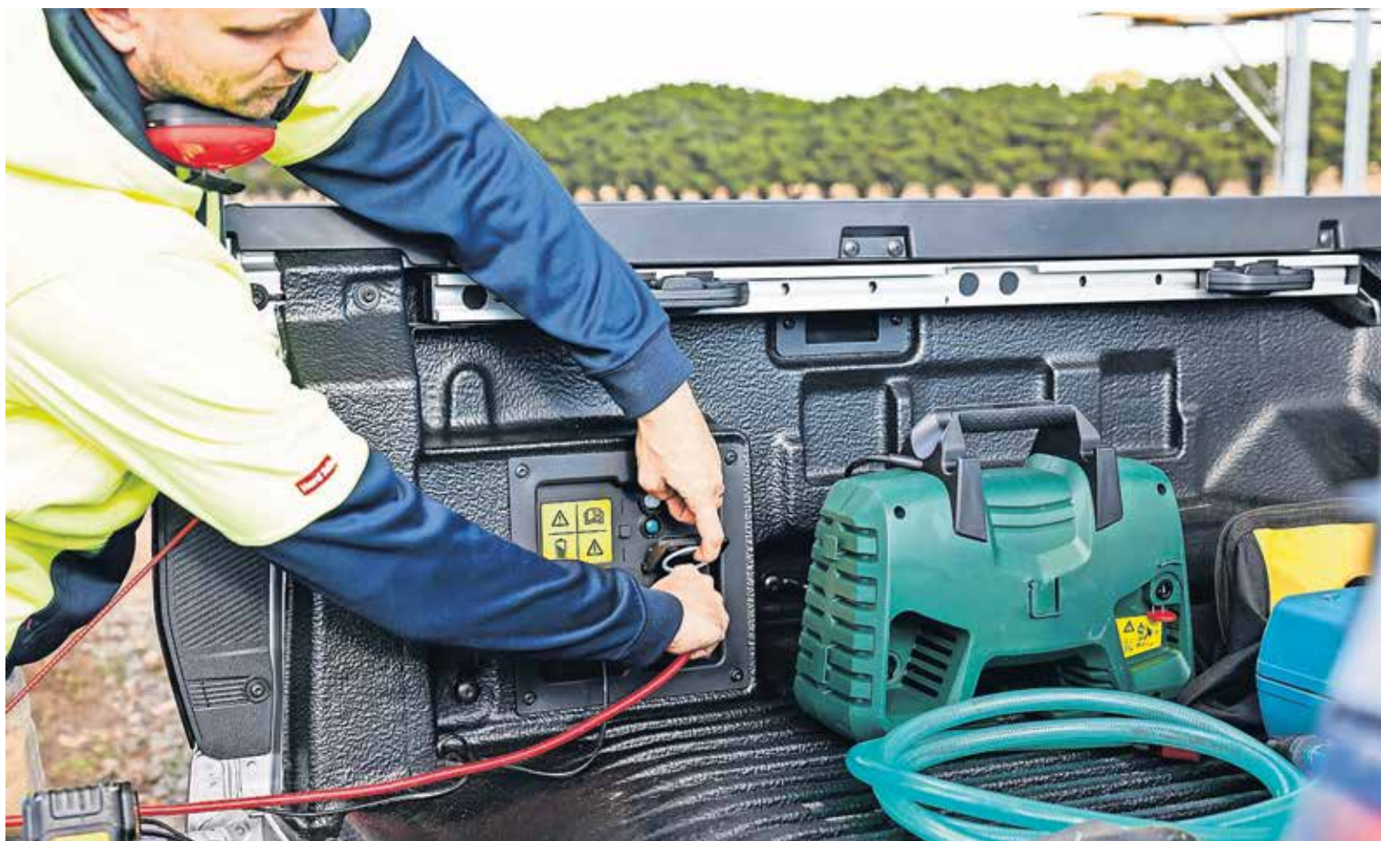
The ability to use a PHEV's battery as an additional power-source on work sites is a game-changer.
