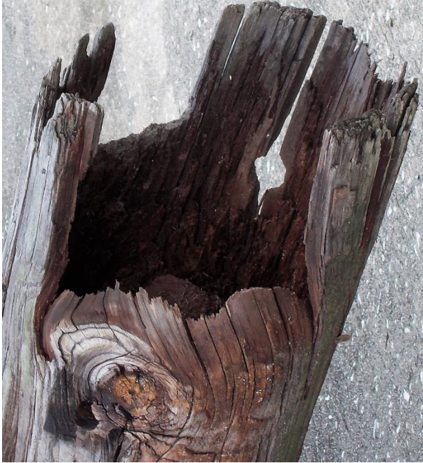
Old Creosote removed from the field, hollow top finally gave way.
