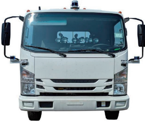
Figure 2 Illustration of the sensors layout of the truck.
