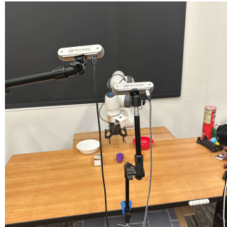
Figure 7: Camera positions for view invariance: old (right) and new (left).
