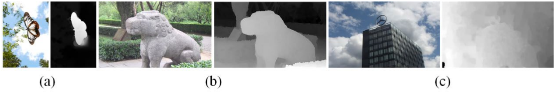
Fig. 3-2 Different qualities of depth maps. (a) Good depth map, \lambda_d = 0.8014 . (b) Common depth map, \lambda_d = 0.3890 . (c) Poor depth map, \lambda_d = 0.0422 .
