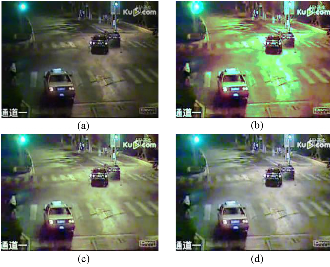
Fig. 5. (a) Original image. (b) Image enhanced by the piecewise strategy without constraint factor-based strategy. (c) Image enhanced by the piecewise-based strategy with constraint. (d) Image enhanced by the factor-based strategy. Best viewed in color.
