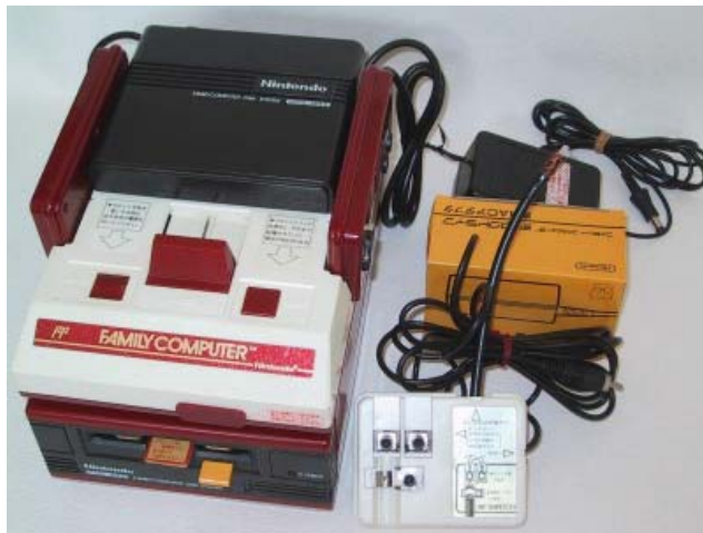
Figure 4-5. Famicom attached to Famicom Disk System [28].
