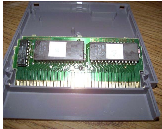
Figure 4-4. Inside a NES cartridge [38].
