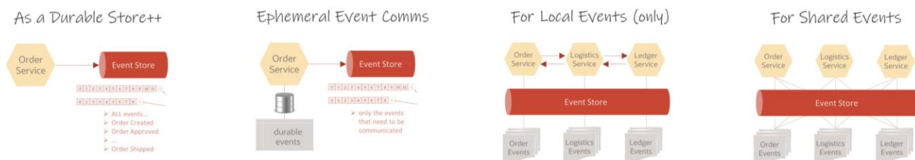
Figure 35: Differing ways that Event Sourcing patterns are used with microservices architecture
